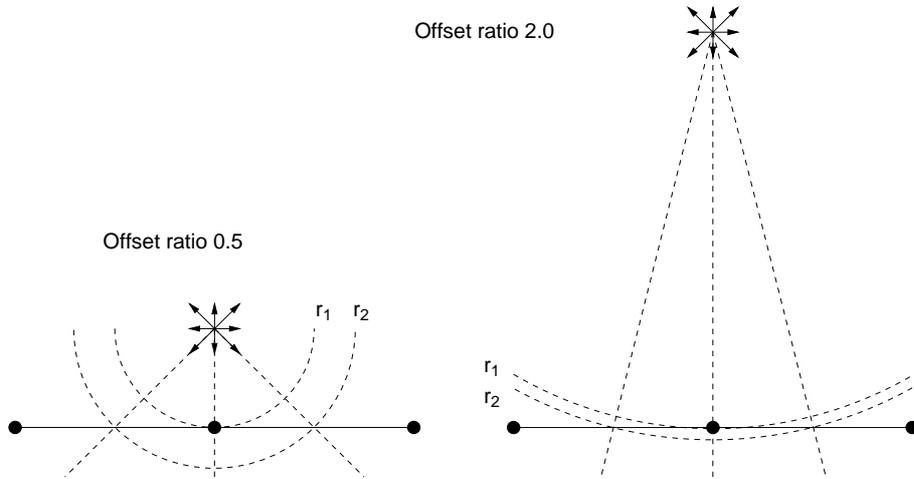
Figure 1: Diagram showing the effect of offset ratio on the accuracy of the boundary condition in the neighbourhood of a collocation point.
