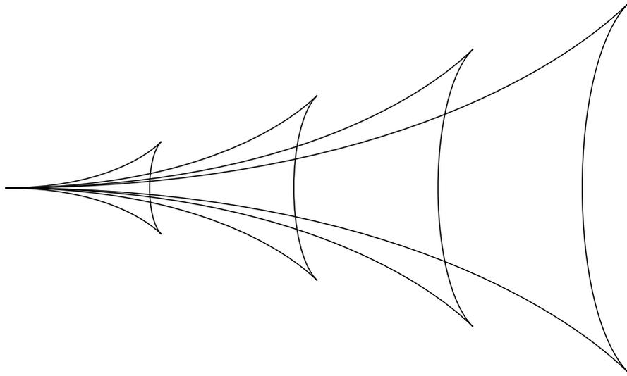
Figure 2: Schematic showing transverse and divergent waves within a typical ship wake.
