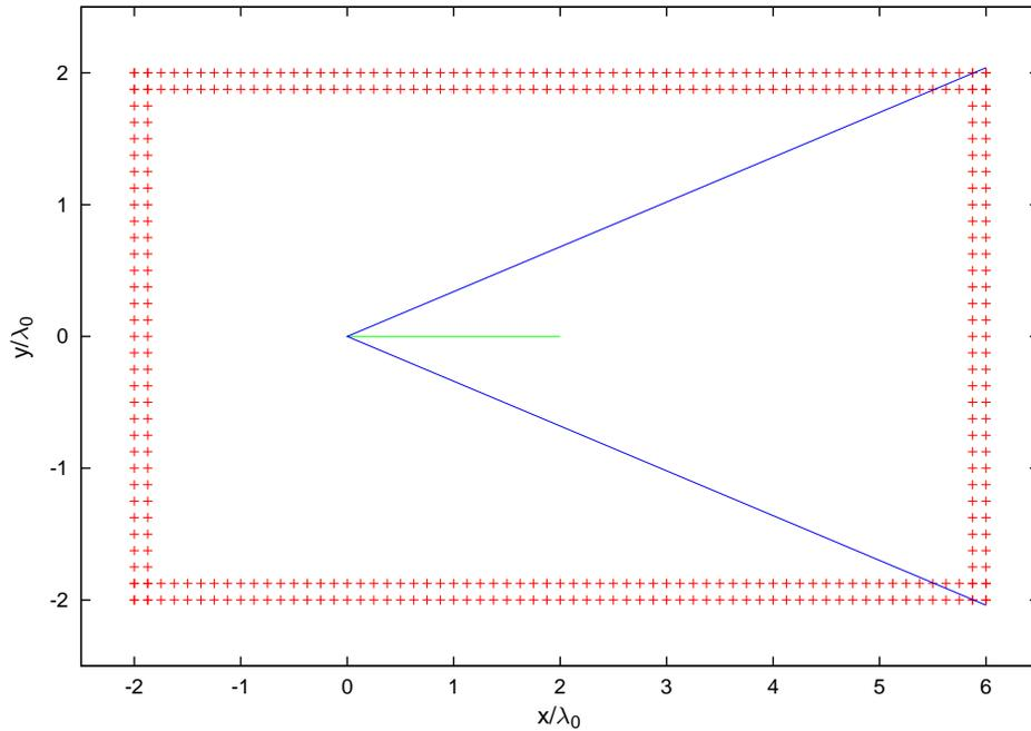
Figure 3: Layout of free-surface collocation points, showing length, width and resolution of domain, together with location of body and wake wedge.
