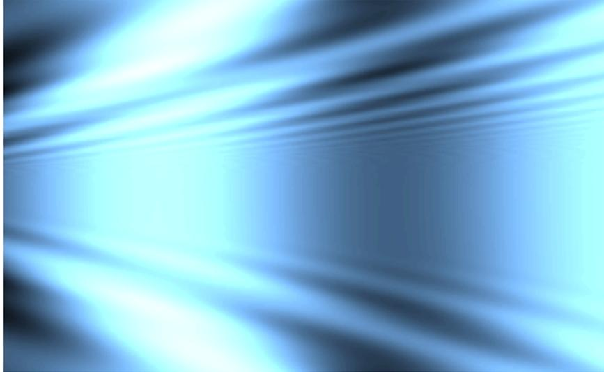
*Figure 2.* Waves made by a destroyer – doubly expanded view. Top half (starboard side of ship) is at zero viscosity, bottom half (port side) is with  $\nu = 0.05 \text{ m}^2\text{s}^{-1}$ .
