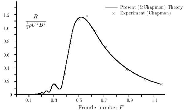
Figure 1: Comparison between theory and experiment for wave resistance of a parabolic strut.
