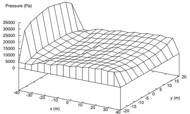
Figure 15: Pressure on flat plate
