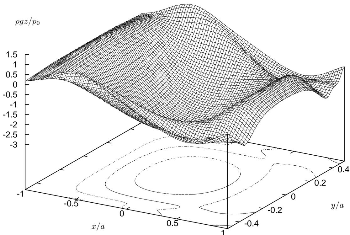
Figure 10: Elevation beneath the tandem pressures of Figure 9.
