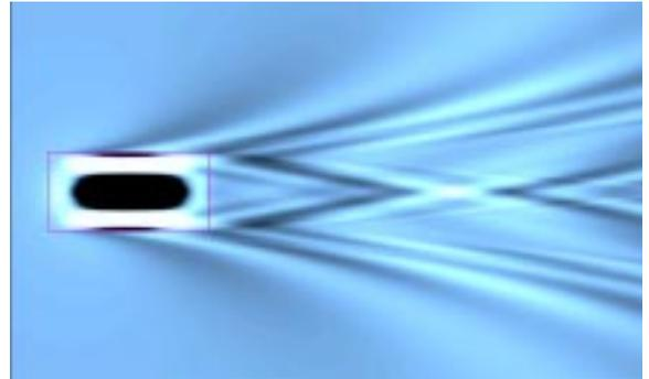
Figure 13: Wave pattern for unconstrained pressure.
