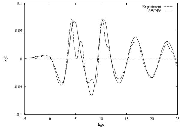
Figure 3: Comparison between SWPE computations for a ship model as in Figure 2 and “Wake-Off” experimental measurements along a cut parallel to the ship’s track.
