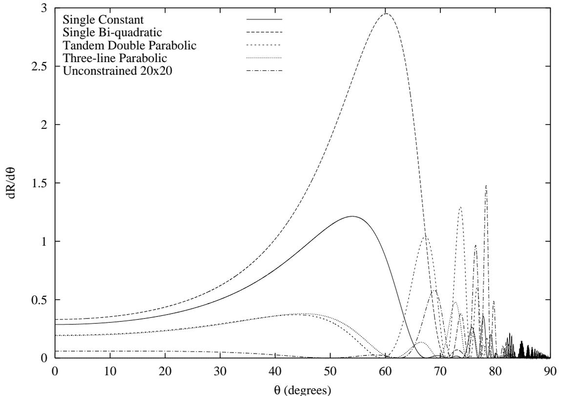
Figure 14: Free wave spectrum for various arrangements of pressure patches.
