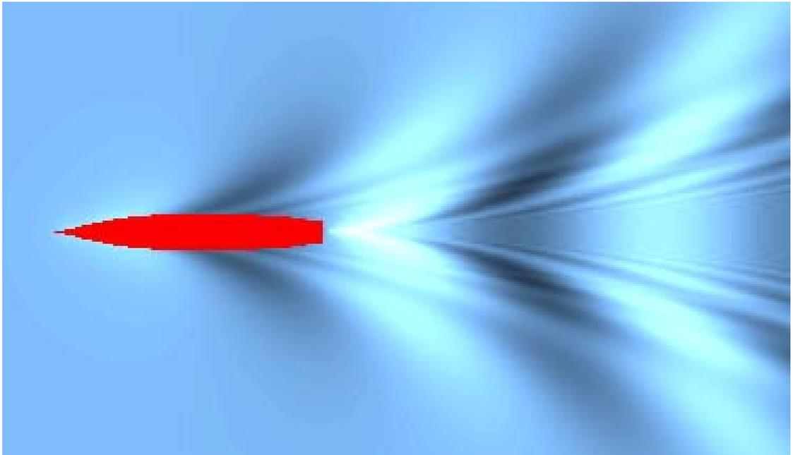
Figure 2: Computed wave pattern for a DDG51 ship at 30 knots.
