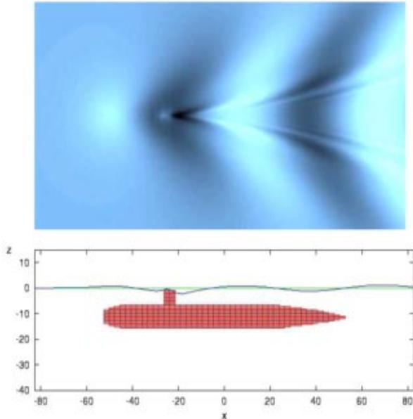
Figure 6: Wave pattern for a submarine.
